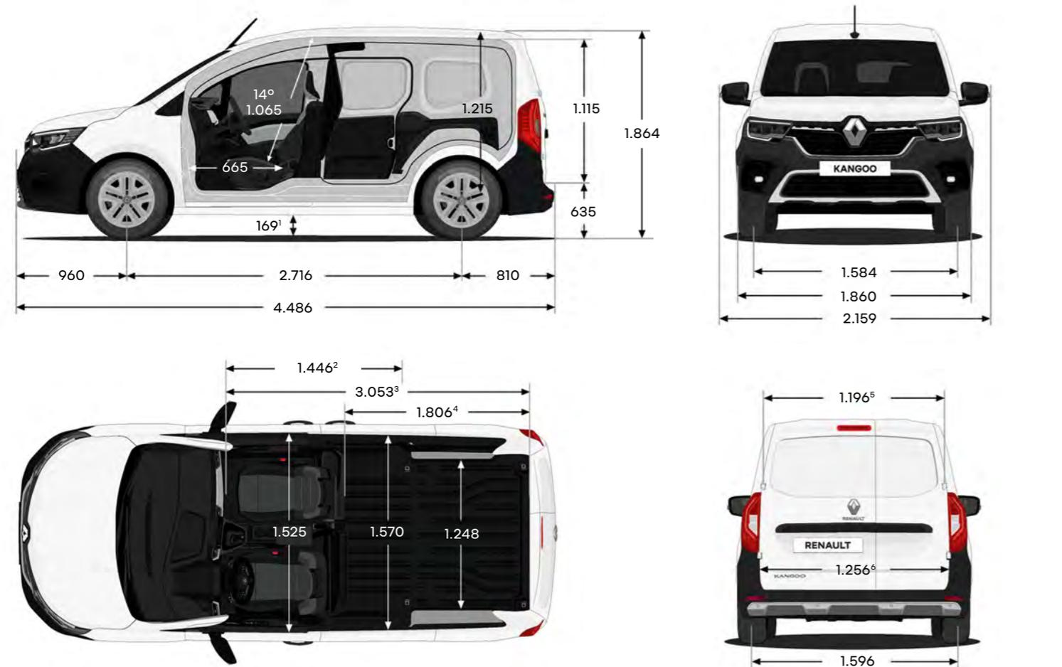
(Abmessungen in mm)
